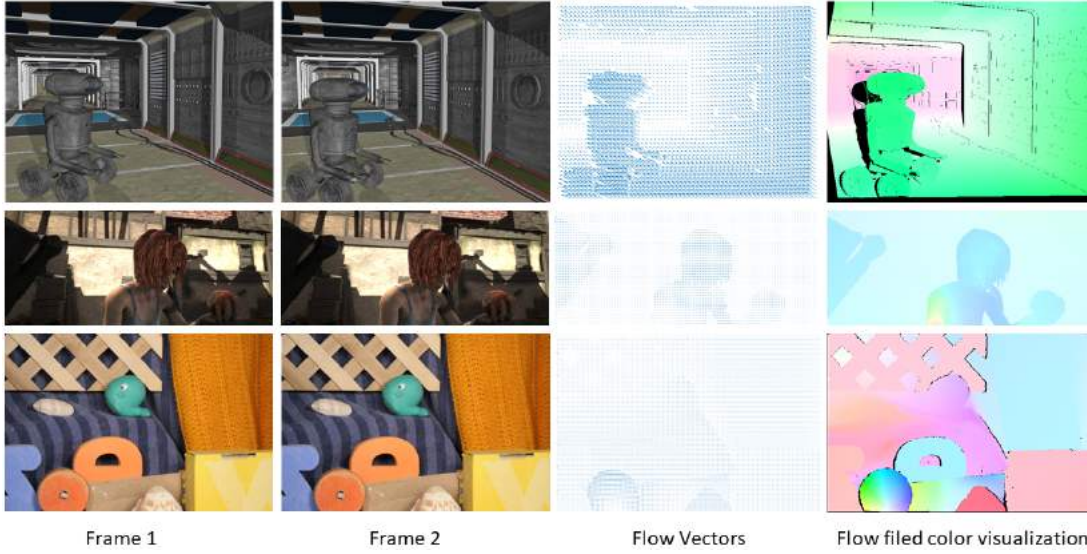
Figure 1.4: Illustration of optical flow. Optical flow is defined as a dense pixel-wise movement between two consecutive frames.
