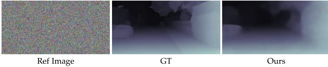
Figure 10.7: Qualitative Result on the Random Dot SfM Dataset. Our method is able to recover structure information from random dot image pairs, which indicates that our method does not rely on semantic contents or image priors.
