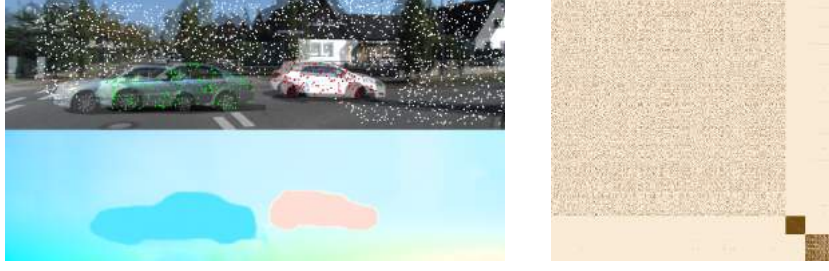
Figure 9.1: Motion segmentation and affinity matrix (constructed from \mathbf{C} ) visualization. The scene contains three motions annotated by three different colours: the ego-motion and the two cars’ movements. On the right, we show a constructed affinity matrix from \mathbf{C} which contains three diagonal blocks corresponding to these three motions. On the bottom left, we illustrate our estimated optical flow and the top left image shows that all these three motions are correctly segmented based on the \mathbf{C} . The sparse dots on the image are the sampled 2000 points that has been used to compute \mathbf{C} . It proves that our Union-of-Subspace constraint can work under multi-body scenarios.
