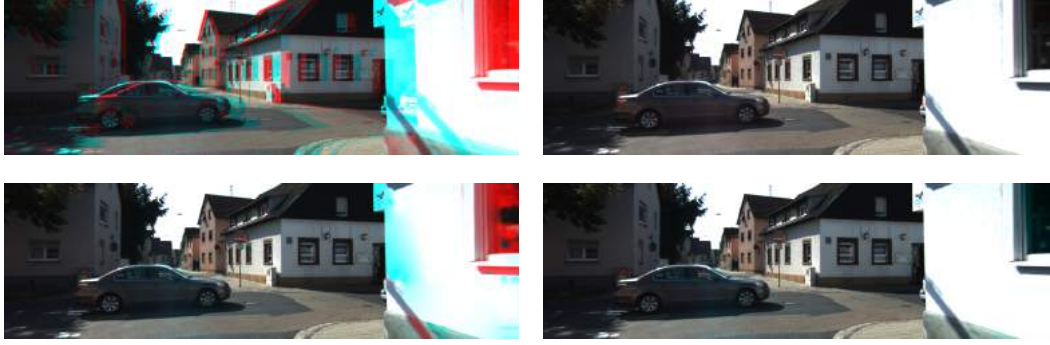
Figure 8.6: Qualitative image separation results on the KITTI-2015 dataset. Top to bottom: Input, ground truth, result from Williem et al. [63], our result. Our method successfully recovers the correct colour of the large textureless region on the right of the image while the other method fails.
